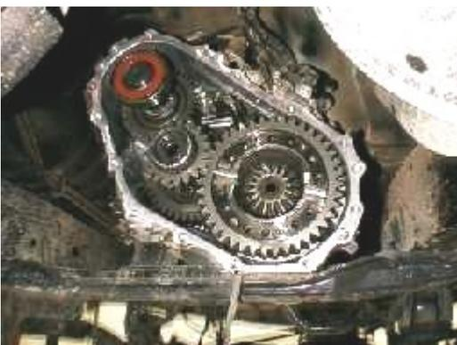
Unbolt rear case, remove gears
